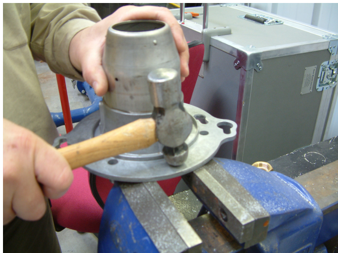
Fig. 5 Punch out the pre-cast profile mounting holes with ball peen hammer.
