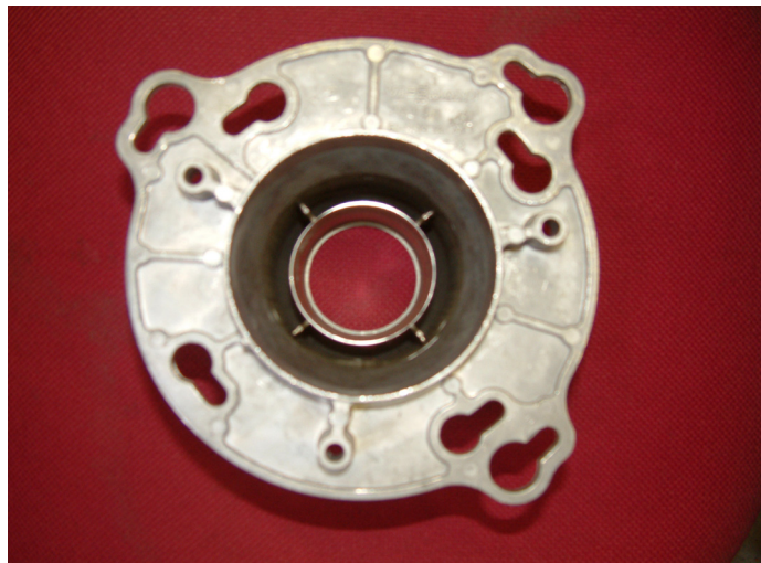
Fig. 8 Mounting flange adapted to four-hole pattern.
