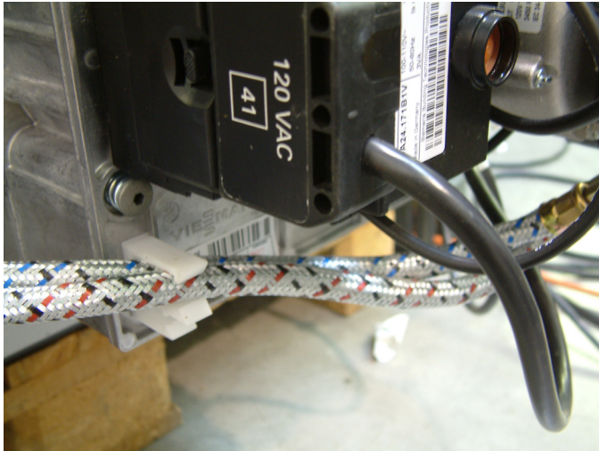
Fig. 13 Route oil hoses and power cable into strain relief. Install burner hood.
