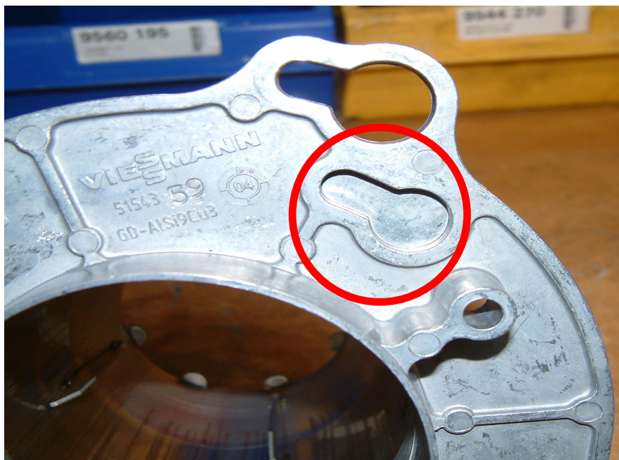
Fig. 4 Punch or drill out the pre-cast profile mounting holes with ball peen hammer and finish the holes with round file.
