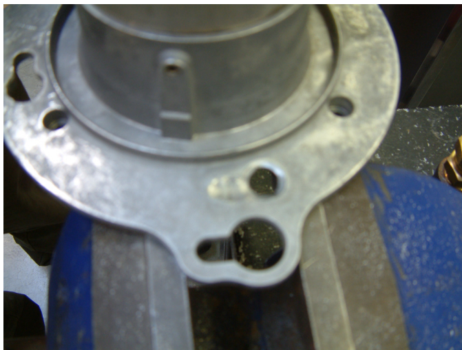
Fig. 6 Broken pre-cast hole
