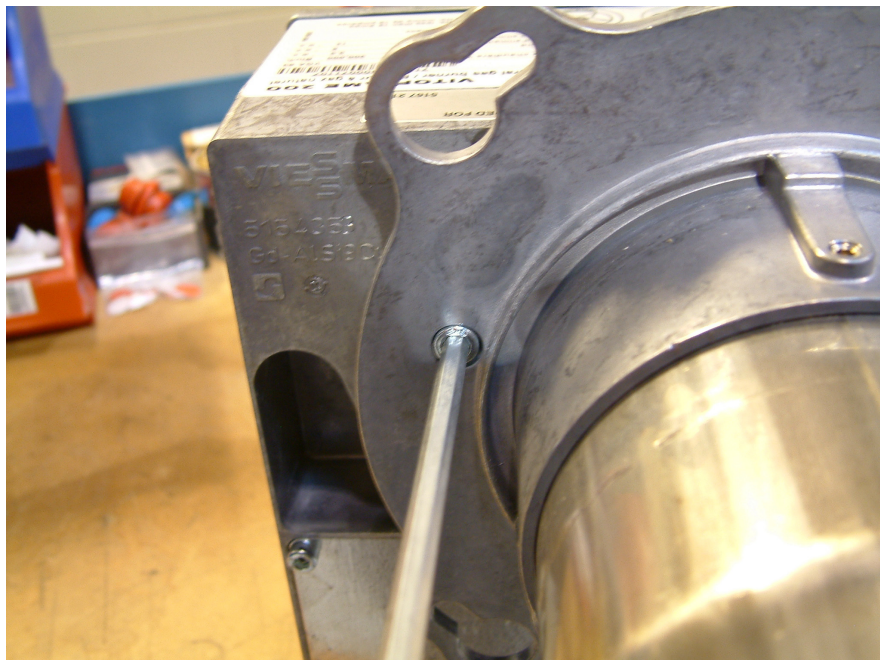
Fig. 3 Remove three bolts and remove mounting flange with blast tube.
